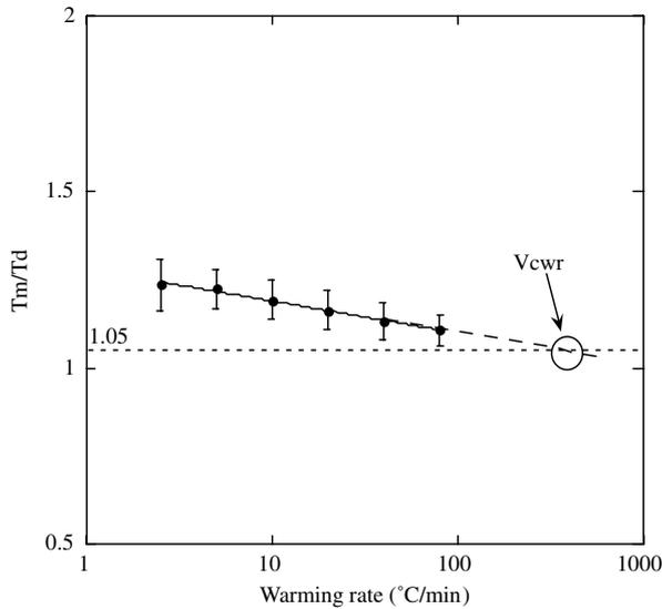
Fig. 4. Variations in the experimental values of  $T_m/T_d$  with warming rate. Isolated points are the mean experimental points with SEM as error bars. The critical warming rate is defined at the warming rate corresponding to  $T_m/T_d = 1.05$ . As usual,  $T_m/T_d$  varies linearly with the warming rate within a very good approximation. The solid straight line is an interpolation by the least square method.
